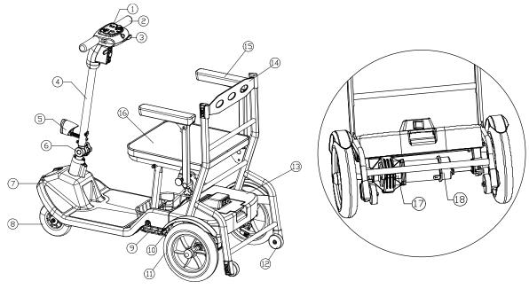
1. Control panel 2. Handgrips 3.Throttle Control Lever 5. Headlight 4. Tiller 6. Tiller adjuster 7. Frame cover 8. Front wheel 9. Storage basket 10. Rear Fender Panel 11. Rear wheel 12. Anti-Tip Wheels 13.Battery box 14. Backrest 15. Arm rest (optional) 16. Seat 17. Transaxle Assembly 18. Manual Freewheel Lever
